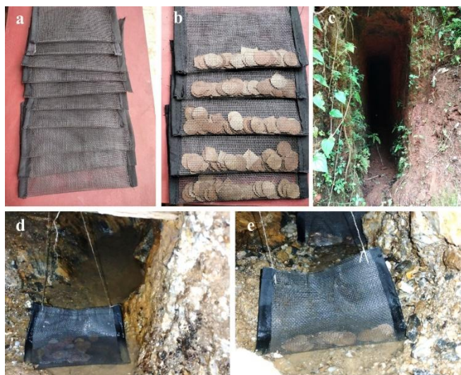
Fig. 2. a, Empty finely meshed litter bags (mesh size, 1 mm); b, litter bags loaded with leaf disks; c, surroundings of the entry point of the cave stream; d and e, submersion of litter bags in the cave stream.
